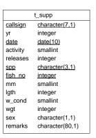
Figure 2: ERD for supplementary data within the tuna database.
